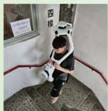
A staff member used a scanner to scan the stairwells of a building. It only took about 15 minutes to complete the scanning of the entire public area of the building.
